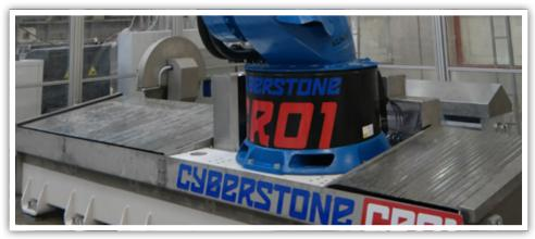
**MONOBLOCK FRAME:** normalized structure in galvanized steel, sandblasted and painted with 3 coats of paint, equipped with rotating table of 1400 mm diameter with aluminum top. It does not require concrete foundation under the floor level. Dimensions 5770 x 2266 mm.
