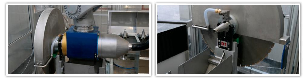
**REVOLVING PLATFORM:** Turntable with interpolated axis, made of steel with aluminum surface, capacity up to 15000kg. Table diameter 1200 mm - Max load diameter 2000 mm.
